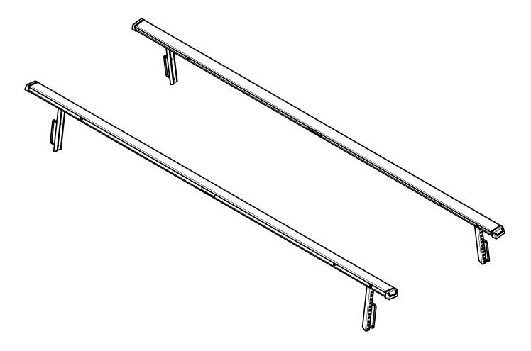
This new bunk assembly is designed to be a full replacement for the carpeted wood bunks, and consists of an aluminum extrusion with a vinyl covering to protect your boat. It is designed to give the same flex and support as the carpeted wood bunks.
