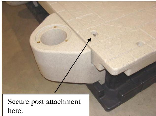
3. Insert flag pole sleeve into the opening on the dock post attachment. Secure with the 3/8 x 1 1/4" bolts and 3/8 washers. Insert flag pole into the sleeve. Will fit flag poles up to 2 1/2" outside diameter.
