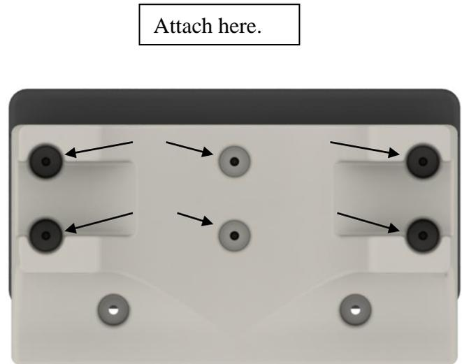
2. Attach the outer pylon hoop to the t-plate and inner hoop assembly using the 1/2 x 8" bolts and washers.
