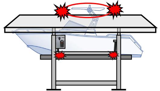
**AUTO-RUN MODE – NOT PERMITTED** DO NOT enter Auto-Run mode if the upper limit is set with a lowered Tower or Bimini. User may forget to lower Tower or Bimini and the motor will NOT STOP. Collision & damage will occur at user's expense.
