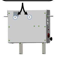
New relay should be mounted horizontally inside of box as shown. Fasteners provided.
