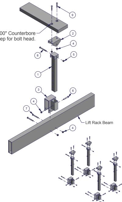
Note: The head of the bolt must go into the counterbore of the pre-drilled holes to avoid damage to the bottom of the watercraft. On 11ft bunks the holes are located 11.25" from one end and 23.25" from the other end and 3" apart vertically. On 14ft bunks the front set of holes are located 20.75" and 25.25" from the end. The rear set of holes is located 20.75" and 25.18" from the end.
