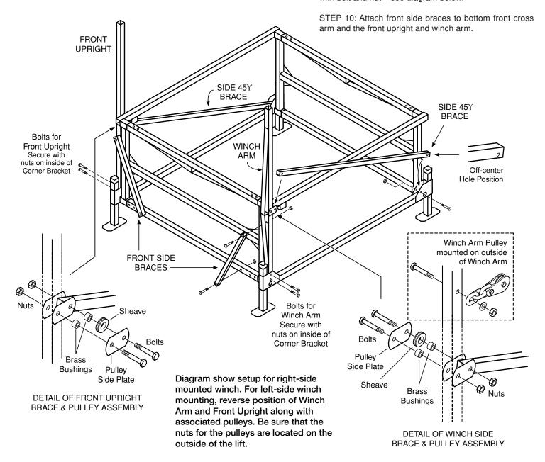
STEP 11: Bolt the complete double pulley assemblies into the pulley boxes on the pull arms, making sure they are slanted toward the **outside** of the lift as shown. Use the two  $^{1}/_{2}$ " x 4" bolts (or  $^{1}/_{2}$ " x  $^{1}/_{2}$ ") with lock nuts. Do not over-tighten. These pulleys must move up and down freely.
