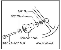
STEP 16: Remove the hex bolt and washer from the threaded shaft on the winch. Grease the threads on the winch wheel so it is able to turn freely. Turn the wheel clockwise on the threaded shaft until it is tight against the winch. Replace washer and hex bolt to secure wheel to winch.
