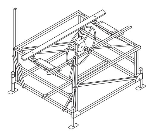
STEP 18: Tighten all bolts and nuts, and make sure that all pulley wheels turn and pivot freely.
