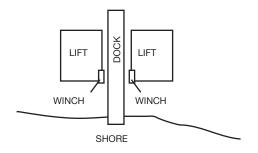
Attach the winch arm to the front corner on the side you have selected for mounting the winch. The winch arm has an identification sticker that gives the model number of the lift. Attach the front upright to the front corner on the opposite side of the lift.
