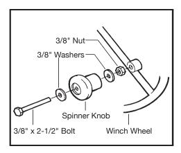
STEP 16: Remove the hex bolt and washer from the threaded shaft on the winch. Grease the threads on the winch wheel so it is able to turn freely. Turn the wheel clockwise on the threaded shaft until it is tight against the winch. Replace washer and hex bolt to secure wheel to winch.
