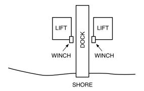
Attach the winch arm to the front corner on the side you have selected for mounting the winch. The winch arm has an identification sticker that gives the model number of the lift. Attach the front upright to the front corner on the opposite side of the lift.
