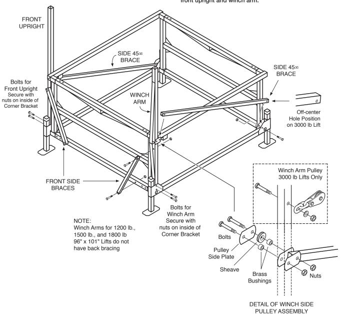
STEP 10: Bolt the complete pulley assemblies into the pulley boxes on the pull arms, making sure they are slanted toward the outside of the lift as shown. Use the two 1/2" x 4" (or 1/2" x 41/2") bolts with lock nuts. Do not over-tighten, making sure the pulleys can move up and down freely.
