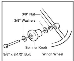
STEP 15: Attach the winch wheel to the winch. Grease the threads on the winch wheel so it is able to turn freely. Turn the wheel clockwise on the thread until it is tight against the winch. Fasten the winch wheel to the winch according to the model number below.
