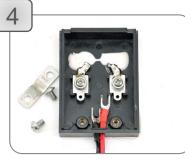
Replace with the new wiring kit, feed fork terminals through hole.
