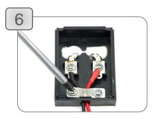
Replace the wire clamp with the hump facing downward
