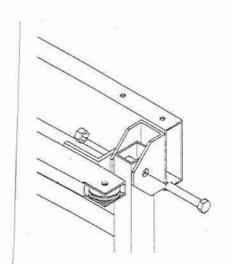
STEP 5: Attach the cradle spreader tubes between the cradles placing the angle caps over their ends.
