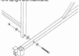
Place a washer under the head of the bolt, under the nut, and between the H Unit and the Mainframe.
