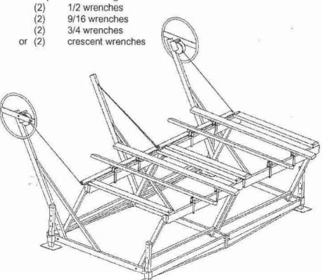
**CAUTION** Do not over tighten the nuts and bolts on your lift. Doing so may cause the lift to fail. When tightening against a tube, tighten until the aluminum just dimples. Lock nuts should be tightened until at least one thread of the bolt is showing through the nut. If you crush the tube, it may crack and fail under normal use.
