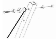
Bolt both cables to the center mainframe
