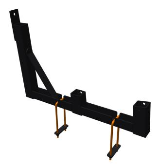
Mount the bunks placing the stop bolt end in it to the entry end of the lift. Place the bunk over the mounting tube and align the hole in the bracket with the hole in the tube. Insert a stainless steel hex bolt thru the bracket and the tube and secure with a flat washer and brass
