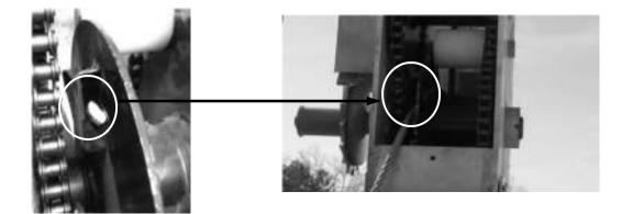
(28) Loop the cable and push the end into the welded clip on the plate. You can tighten the slack in the loop by pulling down on the cable coming out of the Winch Box.
