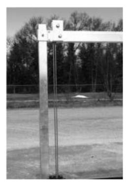
Note: Make sure the cables coming out of the Upper Cable Tube Assembly are running side by side and not twisting around each other. They must be kept parallel in order to raise and lower the lift properly. If they are twisted you may have to remove the cable from the front Twin Beam and re-string through the tube. Please call if you need assistance.
