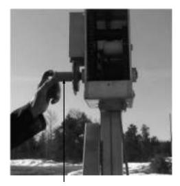
(26) Remove the 3/8"x3/4" bolt and washer from the end of the Winch shaft and take off the thread protective sleeve. The threads will have some grease on it. This keeps the wheel spinning freely. Leave the bolt and washer off for now.
