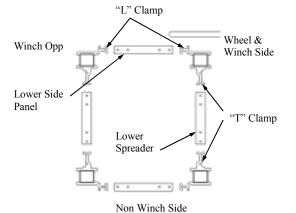
(9) Assemble each corner using the picture as a reference.
