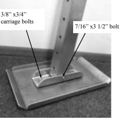
(2) Put the Foot Bracket on the Foot Pad and line up the holes. Put the 3/8" x 3/4" carriage bolts through the Foot Pad so nut will be on the bracket side. Put the leg into the bracket and put 7/16"x 3 1/2" bolt through with nut on end of bolt.
