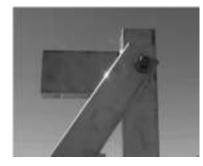
(13) In the upper hole, insert (1) 1/2"x4" bolt, 1/2" washer and 1/2" whiz nut into the Winch Column from the inside going to the outside. Use the washer on the outside of the column. It is not necessary inside the winch box. Take the front cover off the winch box as well as the bottom roller guard plate. Slide the keyhole slot over the flanged bolt. Insert the other bolt through back side of column and attach with nut on winch side.
