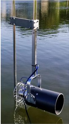
Determine location that will best position the Aquasweep to clear debris, in a minimum water depth of 12". Adjust depth 4" from lake bottom. See back page for additional guidelines.
