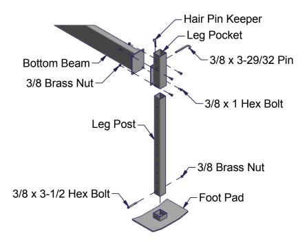
Slide the Lift Side Left and Lift Side Right End Channels on to the two Bottom Beams. Place the Lift Sides on the Bottom Beams so the bolt holes match - as shown. Secure each Lift Side to the Bottom Beam Front using two 3/8 x 3 Hex Bolts and two 3/8 Brass Nuts. Secure each Lift side to the Bottom Beam Rear using three 3/8 x 3 Hex Bolts and three 3/8 Brass Nuts - as shown below.
