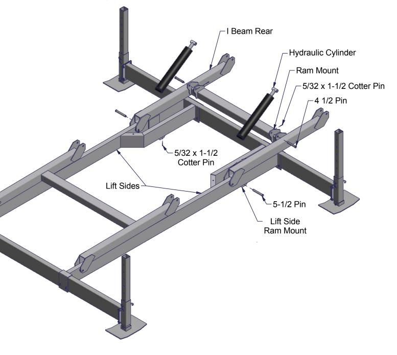
Attach each Rack Side to I Beams using two 4.0 Pins and two  $5/32 \times 1-1/2$  Cotter Pins - as shown. Bend cotter pins with needle nose pliers after inserted.
