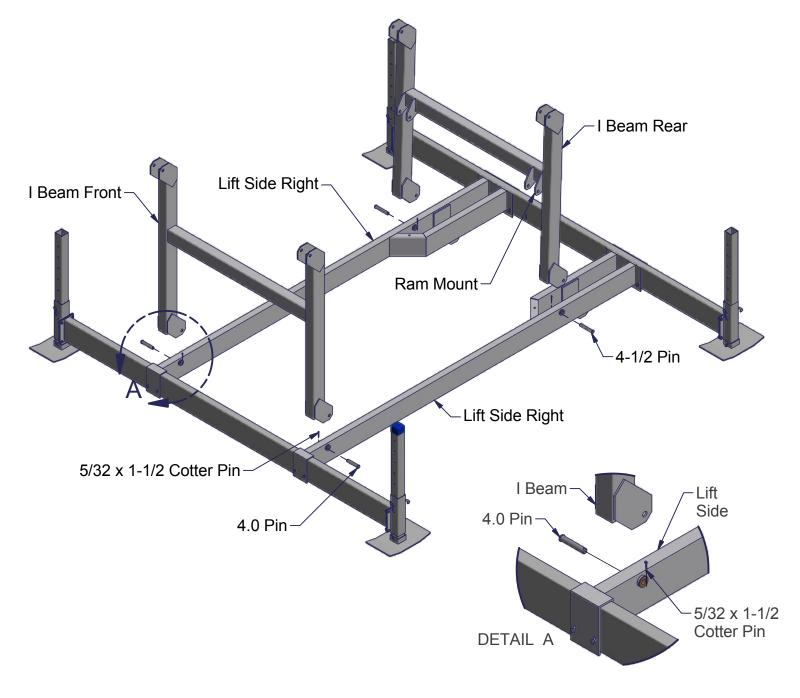
Pin the base of each Hydraulic Cylinder to the Lift Side Ram Mounts using one 5.0 Pin and one  $5/32 \times 1-1/2$  Cotter Pin in two places - as shown. Bend cotter pins with needle nose pliers after installed.
