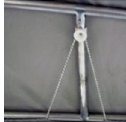
Hook the center bungee up over the canopy cord spool hook located at the top of the 20 1/2" canopy spacer tube. Then hook over the canopy cord spool hooks at the top of the 12 1/2" spacer tubes. Once they are hooked, then hook over top of the canopy cord spool hooks on the 19" spacer tubes.
