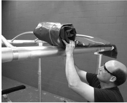
Remove the vinyl cover from the box. Unroll the vinyl cover down the side frame as shown. When completely unrolled, unfold the cover across the canopy bows and pull down over the framework.
