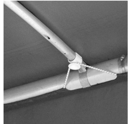
Starting at the middle of the side frames front to rear, pull the bungee cord on the sides of the canopy cover over the top side of the canopy cord spool hooks. Alternate from side to side of the canopy so the cover stays centered on the frame. Continue until they are all attached.
