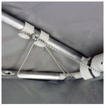
The bungee cords are manufactured to the correct length before they are installed in the cover at the factory.
