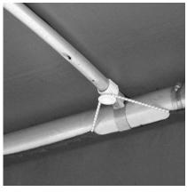
Starting at the middle of the side frames front to rear, pull the bungee cord on the sides of the canopy cover over the top side of the canopy cord spool hooks. Alternate from side to side of the canopy so the cover stays centered on the frame. Continue until they are all attached.
