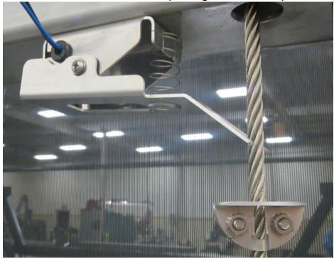
limit switch is installed and the jumper wire is installed. Pull the plug apart, slide one side in until a connection is made then tap other connection 10 times.
