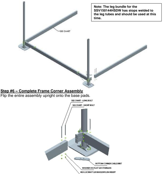
Locate the long bolts and the bottom corner cable bracket. Insert the long bolt with a flat washer thru the second hole from the post, thru the frame tubes and then thru the corner cable bracket on the bottom as shown. Secure with a flat washer and brass lock nut. **Do not tighten**.
