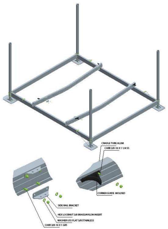
For the 4000, 5000, and 6000 lb. models insert a carriage bolt into the corner guide as shown and slide the head into the top slot in the cradle tube. Secure corner guide with a flat washer and lock nut. Do the same on the other three corners. Slide two carriage bolts into the top slot
