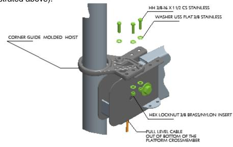
The following picture shows the position of the level cable as it comes over the pulley in the cradle tube and out the bottom to go to the cable mounting bar attached to the corner of the lower frame. Note the other two holes on the end of the cradle tube. These will be used later to attach the cables coming from the bottom of the lift tube.
