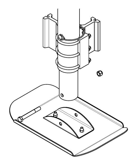
Note that the bolts (1/2-13 X 4 1/2" HC Stainless and Brass lock nut with nylon insert) should be inserted in the same direction as that of the u-bolt. Repeat this process on the remaining legs.
