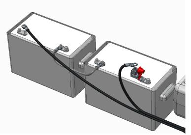
Connect the battery cable from the battery bank to the motor battery cable.
