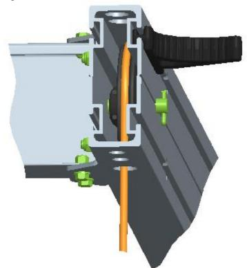
Step #9 – Attach the Level Cable
