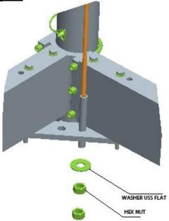
Attach the level cable as shown inserting the cable into the hole <u>closest to the sideframe</u> and securing with a flat washer and 2 brass hex nuts (see chart on page 12 for hardware sizes). The first nut will be run to the bottom of the threads and the second run down and secured tightly against the first. Repeat on other level cable.
