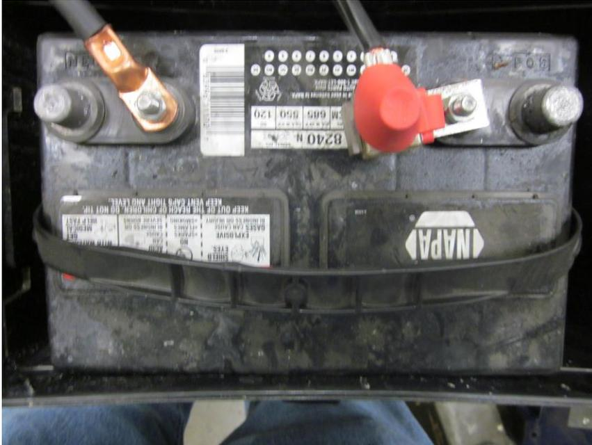
**Step #14 Connecting Battery to 12 Volt Pump**
