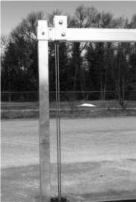
**Note: Make sure the cables coming out of the Upper Cable Tube Assembly are running side by side and not twisting around each other. They must be kept parallel in order to raise and lower the lift properly. If they are twisted you may have to remove the cable from the front Twin Beam and re-string through the tube. Please call if you need assistance.**
