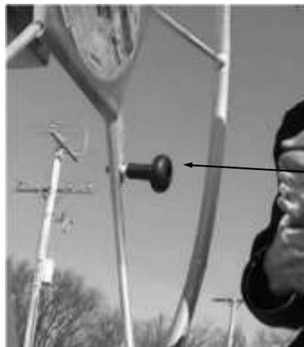
**(31)** Put a 3/8"x2 1/2" bolt through the knob and spin on a 3/8" whiz nut. Don't spin the nut all the way to the knob or else it won't turn freely, leave a small gap. Put the rest of the bolt through the hole in the wheel plate and put a nut on the back side. Use an open end 9/16" wrench to hold the nut by the knob and tighten the nut on the back side of wheel plate.
