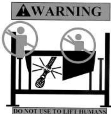
Additional warning sticker is placed on the winch column and on interior of the lift as a reminder of the danger. The boat lift is not meant to lift humans which means the guides on also. The cable can break unexpectedly so keep that in mind and don't allow swimming near or under the lift also.
