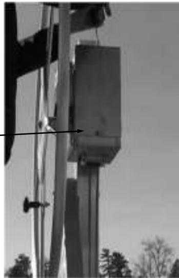
**Note:** Cable life can be extended up to 3 times longer by regular lubrication of the Winch Cable. Don't let out son much cable that it goes slack as it can get caught in the winch gears
