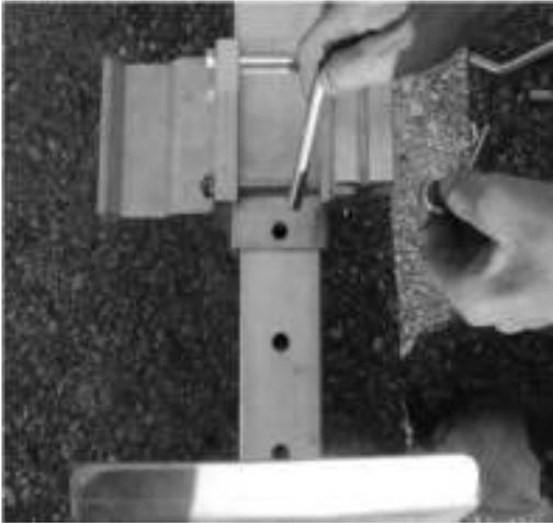
**(5)** Insert the 7/16" leg pin into the 3rd hole up (approx). This will give you room to work under the clamps. You can adjust after hoist is complete if necessary.
