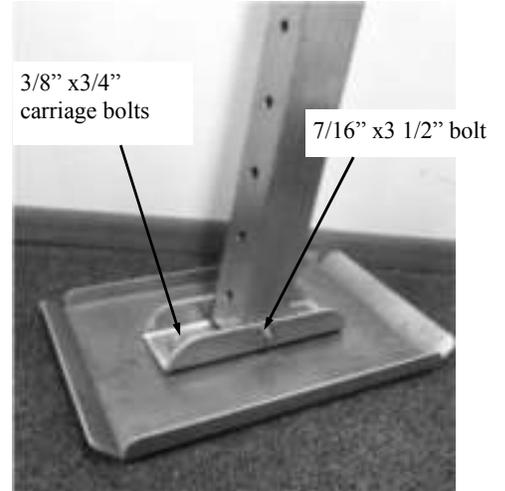
(1) Start by finding the Foot Pads, Foot Pad Brackets and Legs that go together. You will also need 8-3/8"x3/4" carriage bolts, 4-7/16"x3" bolts, 8-3/8" whiz nuts and 4-7/16" whiz nuts to hold the legs together.
