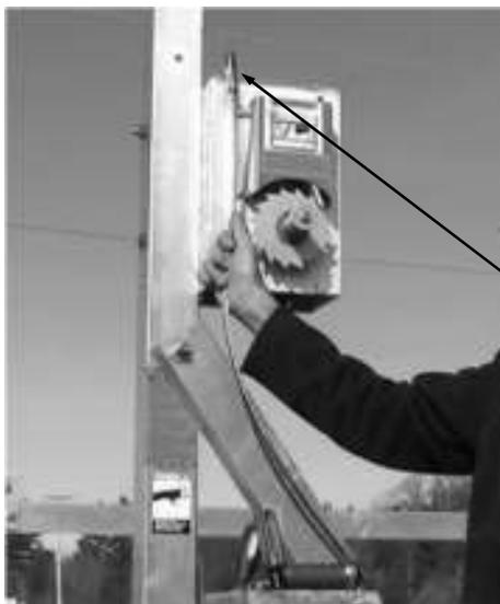
**(25)** Replace the Winch bottom roller cover plate on the winch with 1/4" bolts. Make sure the rollers are positioned closest to the column. The cable coming out of the winch box must be able to move straight up and down. Next pull the cable from the front Twin Beam with the threaded end and insert through the bottom of the winch and up through the hole in the top of the winch. Fasten with a 5/8" washer and a 5/8" lock nut.
