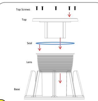
Use Provided wrench and top screws to assembly your light together. NOTE: The seal must be in the correct position before tightening down the top to the base.
