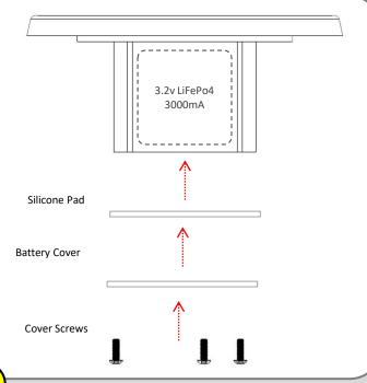
Use the provided wrench and screws to secure the silicone pad and battery cover. Fully tighten screws to ensure the chamber is waterproof.
