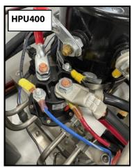
The wires on the new harness go back into the same places as the wires removed and get tightened down.
