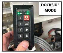
Once the test is completed and the components all work as intended, unplug the main battery power along with the keypad and any extension harnesses and move onto the next step.
