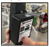
The bottom screw cannot be accessed without the removal of the key switch faceplate. Simply grab the key switch housing by the top and pull away from the ShoreScreen mounting arm. HOLD ONTO THE MOUNTING ARM BEING CAUTIOUS NOT TO DAMAGE IT OR PULL IT AWAY FROM THE FRAME. The light plastic around the bottom screw head should break allowing the key switch assembly to fall free.
