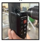
Rotate the keypad assembly out of the way and use a drill and bit to drill a new hole.
