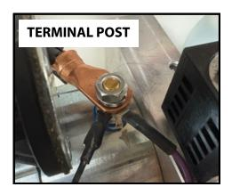
Limit Switch — black/blue wire leading to the external upper limit. Unplug and pull up through the bottom of the box. Additional wires/plugs to note:
