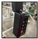
Hold the keypad assembly in place and mark the new top hole location.
