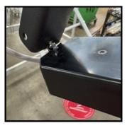
Once the key switch assembly is free, use a pair of snips to cut the wire near the key switch and discard the key switch assembly. Pull the cut wire up and through the hole in the canopy frame and let it hang for now.
