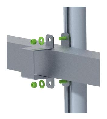
straight vertical and tighten the lock nuts for the lower frame brace and brace tube bracket.
