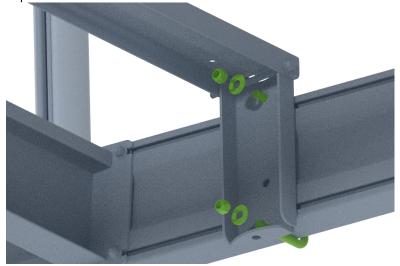
Double check- from inside of the bracket to inside of the bracket on the other side should be about 65"
