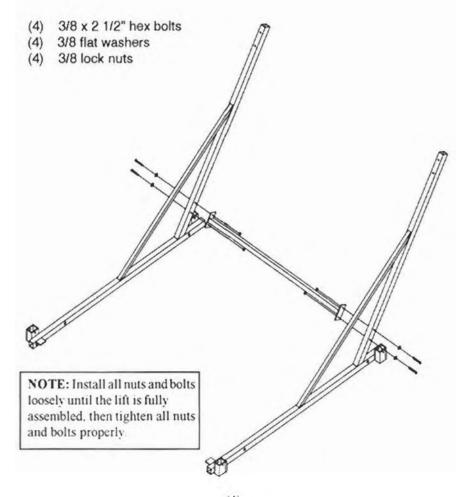
NOTE: The bolts in Step 3 and Step 4 are pivot points which allow the lift to go up and down. These bolts need to remain loose enough to allow the joint to pivot. Do not over tighten.
