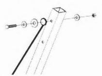
You may now tighten all of the nuts and bolts you have installed except the 1/2" pivot bolts in Step 3 and Step 4.
