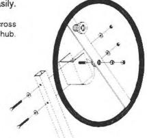
Turn the wheel clockwise until it tightens up against the winch and you hear the braking mechanism begin to click. When you turn the wheel counterclockwise the brake will be released. Make certain the brake is activated when performing the next step.
