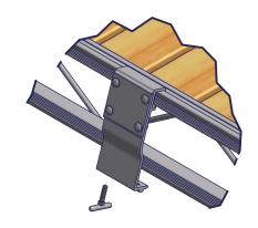
Pivot the top lip of the Accessory Connector Bracket assemby into the Groove on the top of the dock frame - as shown.
