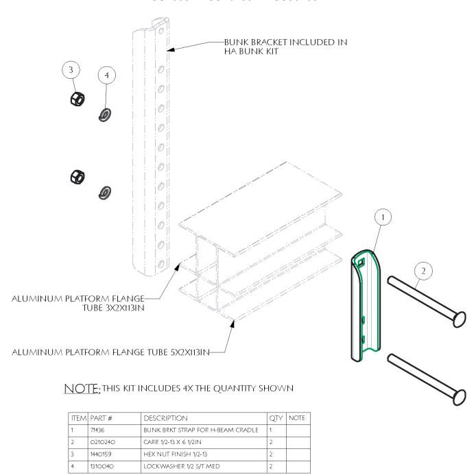
This kit will be mounted with the adjustable bunk brackets to the inside of the platform frame. The bolts will be mounted thru the top hole and the hole will match the size of the H flange tube and secured to the adjustable bunk brackets with lock washers and hex nuts included. Adjust by sliding the brackets in or out and adjusting the hole position on the adjustable bunk brackets.
