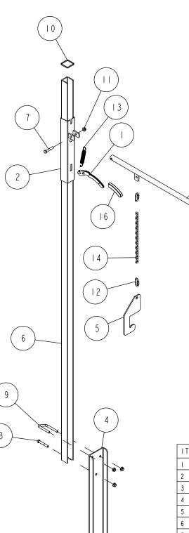
attach by hooking under the cross member. The hook should be placed on the cross member of the dock section with the leg frame attached (The section closest to shore). The hook is shaped so that once it is hooked it will remain hooked until it is removed.
