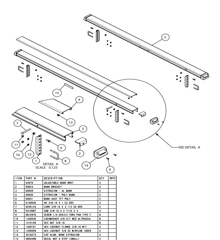
This new bunk assembly is designed to be a full replacement for the carpeted wood bunks, and consists of an aluminum extrusion with a vinyl covering to protect your boat. It is designed to give the same flex and support as the carpeted wood bunks.
