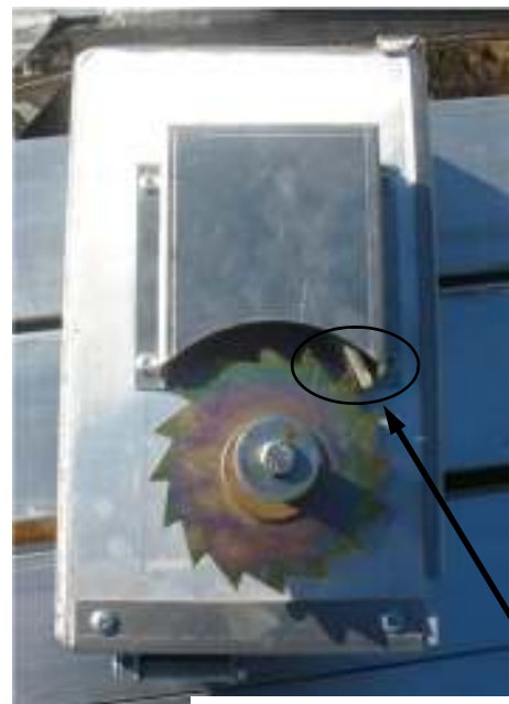
Ratchet, never lift up as this will cause uncontrollable
