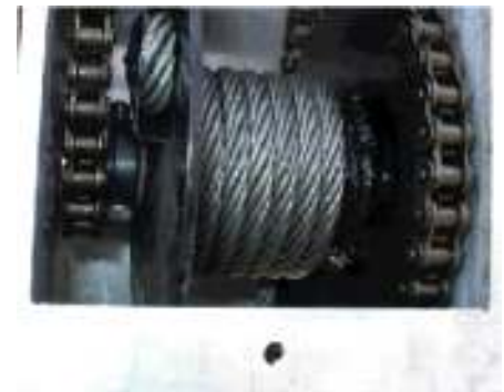
View of how the cable should wind on the drum
