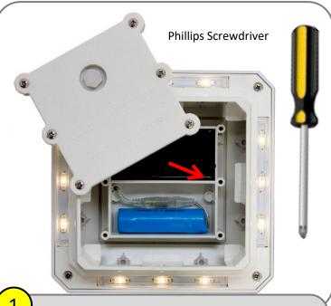
Use a screwdriver to remove the battery cover & connect the battery: **NOTE:** Align the connectors before joining.
