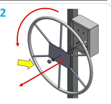
Remove the nut, washer, or bolt holding the wheel on. Turn the wheel counter-clockwise to unthread the wheel from the winch shaft. NOTE: if the wheel is rusted to the shaft try holding the shaft to prevent the shaft from turning while you turn the wheel to break free.
