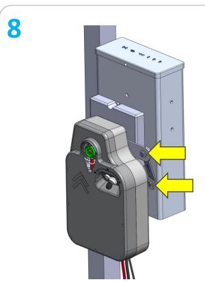
Make necessary adjustments to motor torque arm and hold arm positions then tighten all bolts & nuts securely. Reinstall rubber cover
