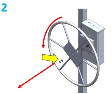
Remove the nut, washer, or bolt holding the wheel on. Turn the wheel counter-clockwise to unthread the wheel from the winch shaft. NOTE: if the wheel is rusted to the shaft try holding the shaft to prevent the shaft from turning while you turn the wheel to break free.
