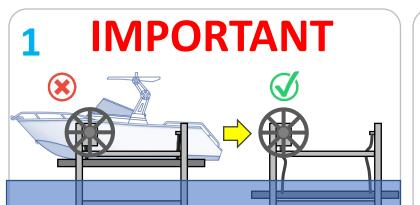
Fully lower the boat lift, remove the boat and any weight from the boat lift carriage. The cable should be slack. Ensure the lift carriage is fully down.
