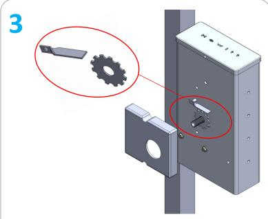
Remove the cover and then remove the break dog and brake disc. These items will no longer be used. Reinstall the cover when finished.
