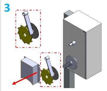
Remove the cover and then remove the brake dog and brake disc. These items will no longer be used.
