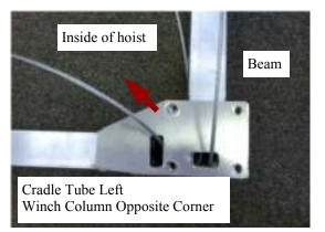
(11) Continue on to the Winch corner. The Cable coming out of the end of the front Beam will not have a threaded end. This end will be connected to the Winch Box in a later step. The cable coming out of the Left Cradle Tube will have a 3/4" button end and will go down to be attached to the corner plate on the lower frame.
