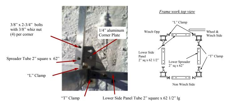
(4) To 'square', or tram the hoist you will need to measure the distance between each Column from inside corner to inside corner as shown below. You may need some help to hold the tape measure. If the two measurements are not equal you can push or pull on the Columns to adjust them accordingly. Once they measure equally go ahead and tighten the bolts and nuts that connect the aluminum corner plates that were assembled in the previous step. See picture on right.
