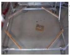
(7) Lay (4)  $4 \times 4$ 's or any 4 equal size boards diagonally across each corner. This will make it easier to put the lift carriage together in the next step.
