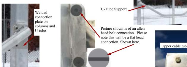
(6) Locate the upper cable tube which is 2" square x 70" long, (4) upper cable tube brackets, (6) 3/8" x 2-3/4" bolts and (6) 3/8" whiz nuts. Hold the tube up at the top of the non winch columns. Get (2) of the upper cable tube brackets and a 3/8" x 2 3/4" bolt, placing one bracket on either side of the tube and align bolts holes. Push the bolt thru to the other side, facing out. Place the 3/8" whiz nut on loosely, do not tighten. Repeat this for the other end. See picture on right.
