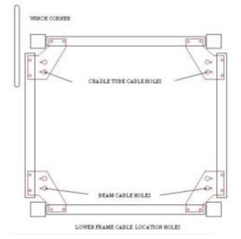
(16) Starting in the Non Winch Column rear corner, pull the two cables with the long threaded end out far enough to reach the holes in the Upper Cable Support Tube. One will be coming out of the beam and the other will be coming out of the cradle tube right. Attach them on the top with (2) 1/2" washers and (2) 1/2" nylon lock nuts. Do not tighten down at this point. Picture below.
