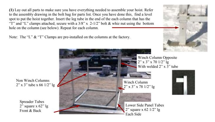
(2) Begin assembling your hoist by locating the columns, side panel tubes and spreader tubes. Start with one of the winch columns, stand it upright and slide the side panel tube over the "L" clamp. The smaller of the two clamps. Put (2) 3/8" x 2-3/4" bolts in the holes. See lower frame top view below.
