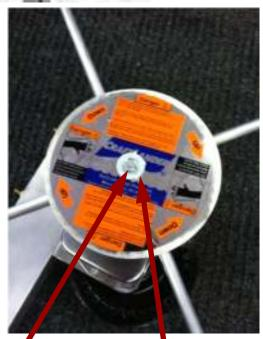
(22) Put the 5/16" hex bolt and flat washer that came in winch box into the winch shaft and tighten. When done there will be a small gap between the washer and the wheel. This allows the wheel to back off the brake in the winch so the hoist will go down. Note: Down is counter clockwise.
