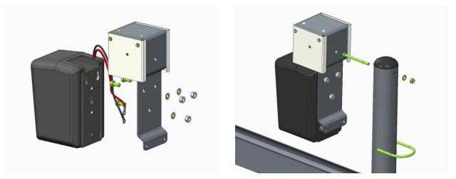
Next, clamp the battery to the corner post as shown.
