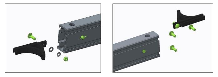
Using those bolts, mount a side rail on each end of the cradle tube as shown. Position the outer edge of the rails at least 3 inches from the end of the cradle tube. It is important to keep this distance equal on all four corners to keep it square. Do the same on the other three corners. **DO NOT TIGHTEN.**
