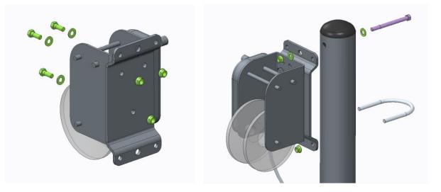
Next, slide on the wheel and spring and tighten the locknut.
