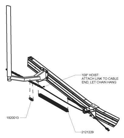
Note: The arms will provide full opening for 132", 120", and 108" hoists, which is 127", 115", and 103" respectively. The retracted opening will be 80", 74", and 68". No adjustment Is necessary.
