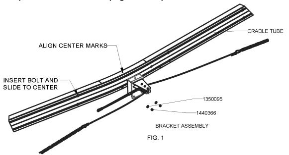
Attach left and right swing arm assemblies as shown in Figure 2. Insert 2 stainless steel carriage bolts into each slot as shown below on each end of the v-frame tube mount the brackets over the bolts and secure with stainless steel flat washers and brass lock nuts. Do not tighten at this time. Repeat on the other side.
